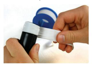
USE TEFLON TAPE FOR PROPER JOINT WITH VALVE. (REFER FIG. FOR PROPER USE OF TEFLON TAPE)
